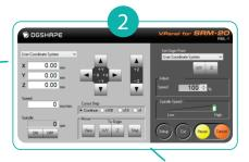
Open V panel for SRM-20 for User Coordinate System for bit's positioning.
