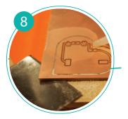
Click [Add] and select the [.rml file] for the circuit's traces. When the [Output] button is pressed, the machine will begin to mill.
